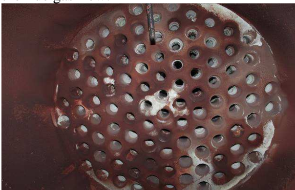
Photo 4. Thick layer of fine deposits on the tube sheet at the first pass flue gas outlet.
