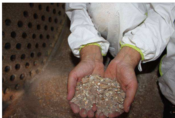
Photo 13. Insignificant quantities of hard deposits on the bottom of the intermediate header, which are systematically removed from the first pass.
