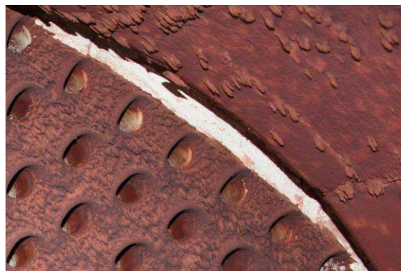
Photo 5. Intermediate header, which joins the first and the second pass of the heat recovery boiler, with its walls covered with deposits.
