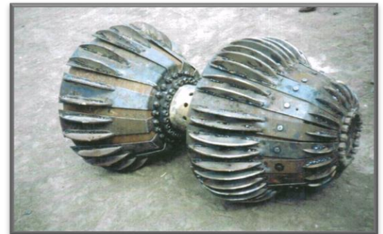
Hydrodynamic cavitation generator HGK 700 for a 700 mm pipeline diameter
